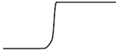
Signal with a short ground lead
